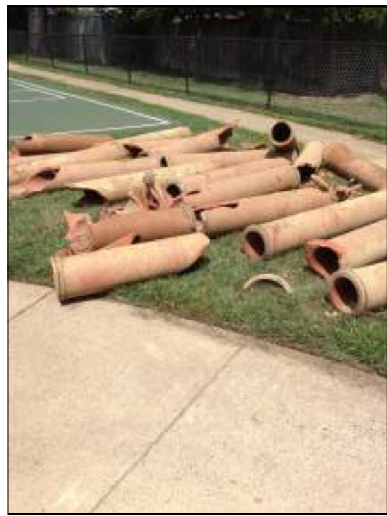
Original Orangeburg pipe, seen above after its removal, needed to be replaced prior to construction of the new tot lot.
