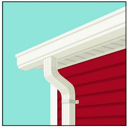
**REPLACEMENT** - The Glen has been gradually replacing (1) its older 2x3 downspouts with harderto-clog 3x4 downspouts and (2) its older, smaller gutters that are attached to buildings by pins with larger, pin-less gutters that rest on PVC rather than wood. These upgrades were part of the roof replacements of recent years. For residents having older roofs, these upgrades have been made on an as-needed basis.
