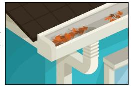
All it takes is a few leaves and twigs that cannot be seen from the ground to block the intersection of a gutter and downspout. A sign that your gutter has been overflowing during storms when you are not home to see it is the presence of vertical streaks running along the length of the gutter.
